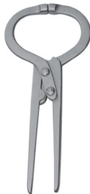
WI-260 Lütje's folding hoof tester, jaw 12 cm, 24 cm, chrome plated
